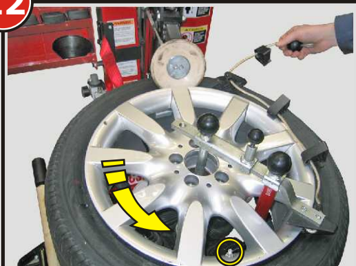
Remove Bead Depressor Tail
